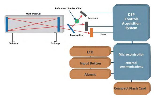
This results in methane detection only and the elimination of false alarms. The laser diode responds faster than other technologies to presence of methane and recovers faster from exposure to high methane levels than other types of instruments. The '46 Hawk's sensitivity and specificity for methane meets or exceeds that of older technologies.
